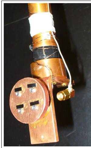
Figure 4.1: Pieces of the sample (glued to the copper sample holder)
